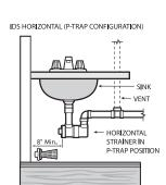
IDS HORIZONTAL WITH ALTERNATE P-TRAP SINK
